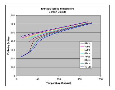
The critical pressure and temperature of  $CO_2$  are  $P_{cr} = 7.38$  MPa and  $T_{cr} = 31.1$  °C.
